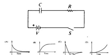
Assume the capacitor  $C$  is initially uncharged. The following graphs may represent different quantities related to the circuit as functions of time  $t$  after the switch  $S$  is closed
