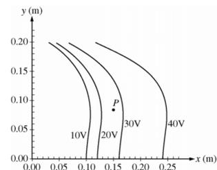
A fixed charge distribution produces the equipotential lines shown in the figure above.
