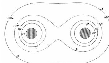
The diagram above shows some of the equipotentials in a plane perpendicular to two parallel charged metal cylinders. The potential of each line is labeled.
