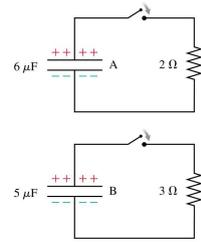
27. The following circuits contain capacitors that are charged to 5.0 V. All of the switches are closed at the same time. After 1 second has passed, which capacitor is charged to the highest voltage?
