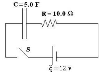
For the RC circuit shown, the resistance is  $R = 10.0 \Omega$ , the capacitance is  $C = 500.0 \mu\text{F}$  and the battery has voltage  $\xi = 12 \text{ volts}$ . The capacitor is initially uncharged when the switch  $S$  is closed at time  $t = 0$ . At some time later, the current in the circuit is  $0.50 \text{ A}$ . What is the potential difference across the Capacitor at that time?
