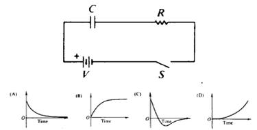
Assume the capacitor  $C$  is initially uncharged. The following graphs may represent different quantities related to the circuit as functions of time  $t$  after the switch  $S$  is closed
