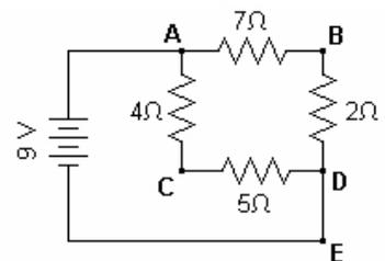
A 9-volt battery is connected to four resistors to form a simple circuit as shown.
