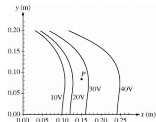
The diagram above shows some of the equipotentials in a plane perpendicular to two parallel charged metal cylinders. The potential of each line is labeled.
