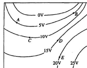
The diagram above shows equipotential lines produced by an unknown charge distribution. A, B, C, D, and E are points in the plane.
