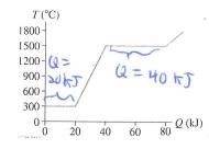
14. An experiment measures the temperature of a 200 g substance while steadily supplying heat to it. What is the specific heat of the substance during the liquid phase? Q = MCST
